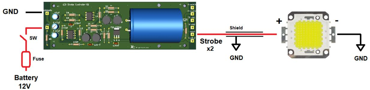
Connect the Strobe output to the LED positive side via shielded cable and connect the shield to ground at one end for each strobe.
